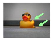
The left image (in Mr. Julian's test) by Z-220 shows that Focus Light and Laser have been exposed on the image. Focus Light exposed on the right side of the subject and the laser on the shoulder. In this case, the camera calculated exposure with Focus Light amount so the image can not be underexposed. If the Focus Light had been turned off, the image should have been underexposed as same as D-2000.
