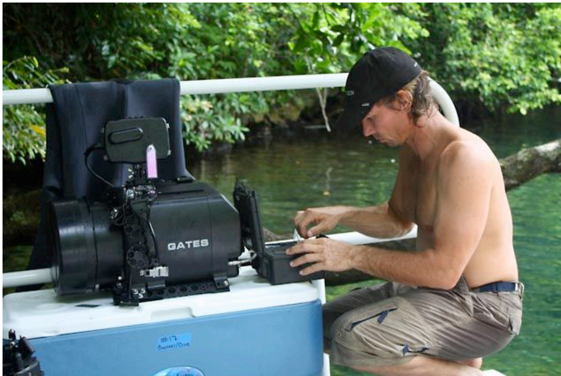
Above: John Friday pulls a vacuum on Deep Red. Note the umbilical connection to the lower right of the housing. Remember to reconnect the valve cover once done!
