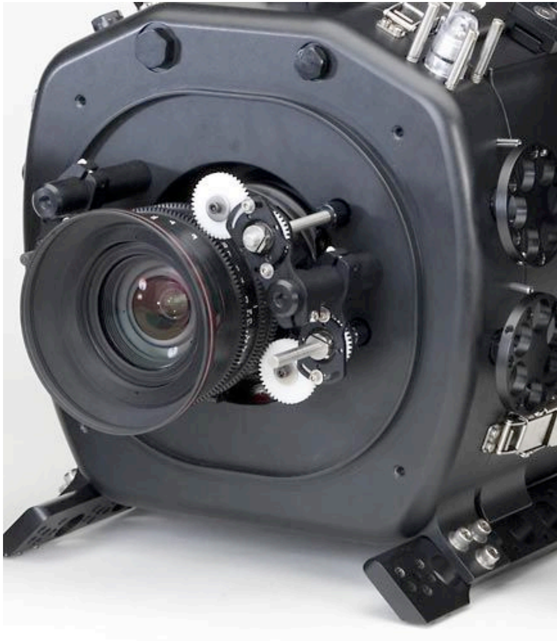
Above: The gearing system developed by the engineers at Gates. Each control mechanism has its own set screws which allow you to position iris and focus gearing at just the right spot. Well thought out and nicely put together.
