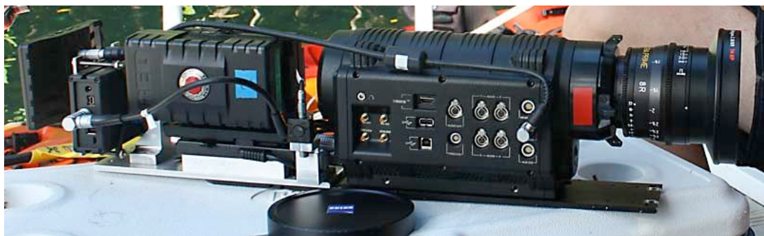
Above: The elongated layout of the timelapse camera meant for an even longer underwater assembly once housing and domes were taken into account.
