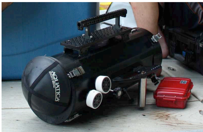
Left: Housing option #3 that started out as an original AquaVideo unit. It has since been elongated so as to accommodate more batteries for longer run times. The impressive workmanship of Mr. Joe Ortega of SL Cine in Los Angeles is very evident.
