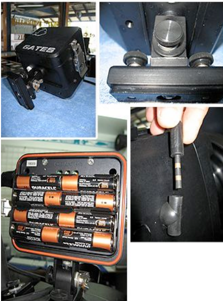
Fig.14 showing the various aspects of the EM419 external monitor including the dovetailed connector plate, the bulkhead connector jack and the internal battery bay. Note that above the battery bay you have the three controls for Brightness, Colour and Contrast. These need to be set when the camera is connected to the monitor via the AV cable once it has been mounted through the bulkhead connection. My housing came with the bulkhead connector already in place hence the lacking of images to show its preparation and mounting. Another note is that I personally feel the monitor lacks contrast and sharpness. This is to be expected when using an SD monitor for an HDV camera.
