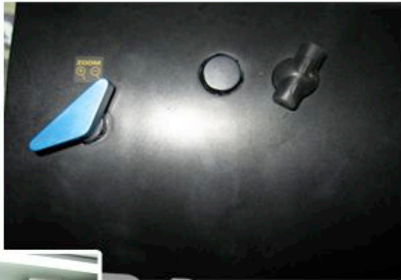
Fig. 6 (Above) Shows the right hand side of the main section. The blue rocker is for Zoom with an optional Video Out (plugged) port and the bulkhead connection for the use of external monitors.
