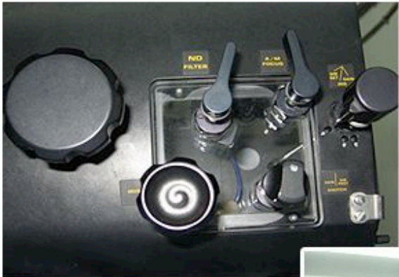
Fig. 4 (Above) Shows the left hand side of the main front section of the housing, the large circular dial at the front being the manual Focus ring. Fig. 5. (Lower) shows the CC flip filter arm control on the front face.
