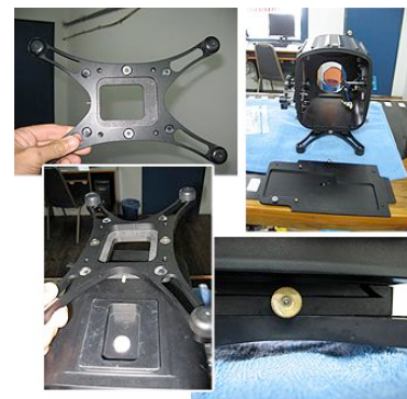
Fig. 11 Shows the base for the housing when using the Fathoms Imaging SWP44. It slides easily into place along the base guide grooves of the housing and is tightened and secured by the brass coloured retaining screw as shown in the bottom right image. When standing upright and with the lens in place, with the lens protective cover on, it offers approximately 1cm (1/3 rd Inch) of clearance to the surface on which the housing is placed. Images to follow.
