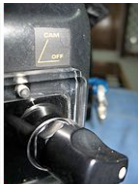
Fig. 8. The On / Off switch on the rear of the unit.
