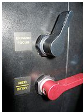
Fig. 9 (Left) Shows the (optional) control for expanded focus and the REC / Standby lever. Above Right shows the eyepiece / viewfinder.
