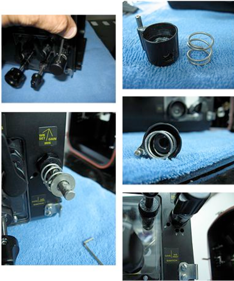
Fig. 10 Shows the steps from top left of how to remove the spring loaded dials. Make sure to keep an eye on the grub screw once removed!! I now know every floorboard in my office personally....you can see how the spring diameter is bigger than the internal stopper of the control dial in the second image down on the right. I placed a washer over the control shaft that would give a better, more secure, base for the spring to rest against. Make sure to re-align the controls before replacing the outer control dial.
