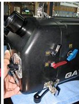
Fig. 9 (Left) Shows the (optional) control for expanded focus and the REC / Standby lever. Above Right shows the eyepiece / viewfinder.
